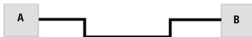
Figure 3 Straight pipe routing between two buildings, with expansion accommodated by Z-bends within the pipeline.
